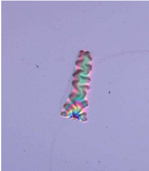
Figure 6.6: A buckled membrane due to the strain from the substrate, shown in this image of the MBE grown membrane after the backside has been etched. When the cantilevers are etched in the ICP this strain will be relieved and the cantilevers will be flat.
