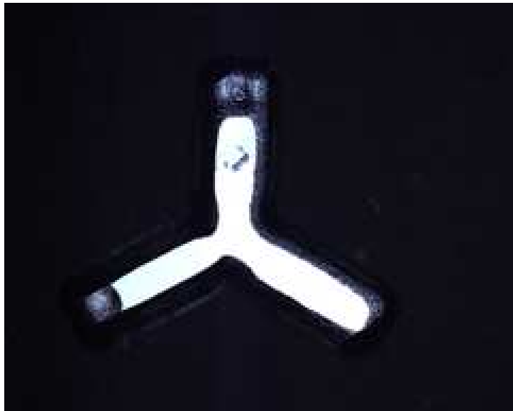
Figure 6.7: Future trap designs might include “Y” junction regions (for a three layer trap, but not a two layer trap). The “Y” shaped backside etch would be complicated by the etching differences between the axis parallel and perpendicular to the substrate flat. By aligning one stem of the Y parallel to the flat and the other stems at a 60^\circ angle, the membrane edges come out straight, similar to figure 6.3
