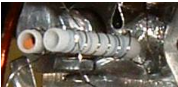
Figure 4.6: Two cadmium ovens, made out of ceramic tubes with tungsten wires coiled around each tube for current heating. The orange material seen on the inside is cadmium oxide. Typically an oven like this would also have a small ceramic aperture at the front to make sure the cadmium oxide does not fall out when the oven is heated.
