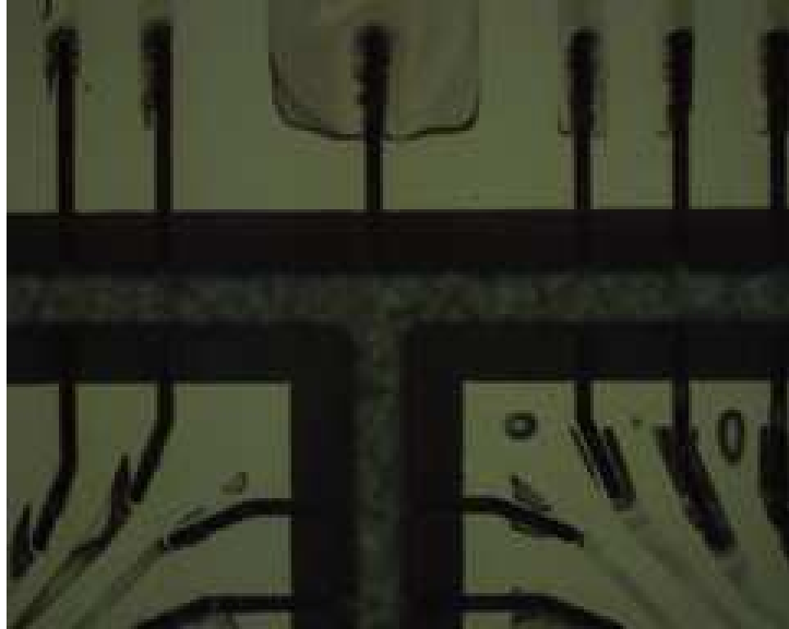
Figure 5.6: T trap photoresist removal; since the photoresist had to stay in longer to develop the edges and cantilevers (you can still see some on the right corner cantilever), some of the photoresist between two wires came off (see the left corner cantilever).
