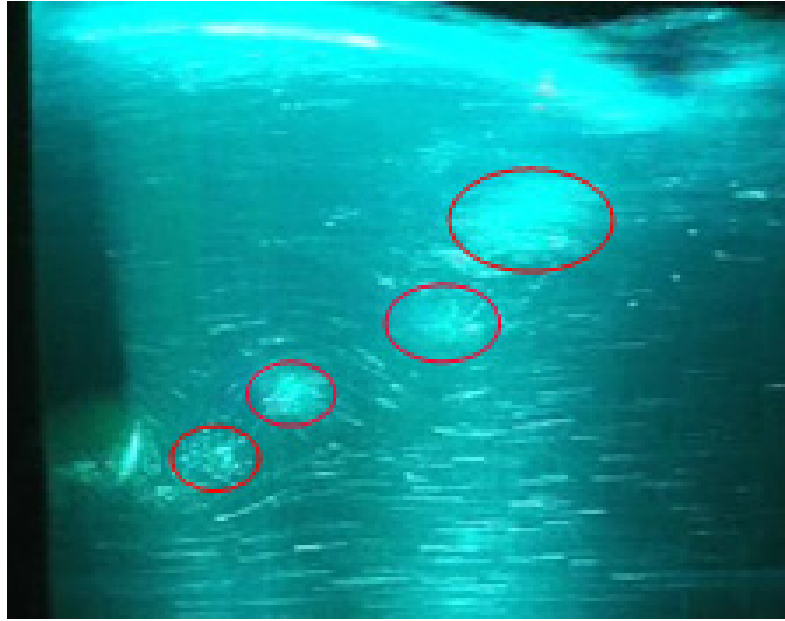
Figure 7.29. Preliminary visualization of the wake of an oscillating cylinder with rough strip showing four vortex structures in one half of the oscillation.
