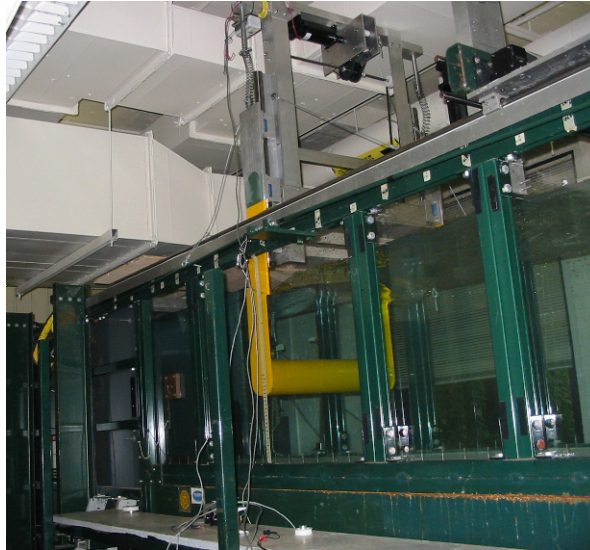
Figure 3.6. VIVACE model in the Low Turbulence Free Surface Water Channel of the Marine Hydrodynamics Laboratory of the University of Michigan.
