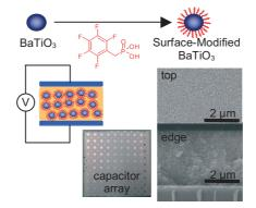
Phosphonic acids act as robust surface modifiers on barium titanate (BT) nanoparticles (NPs) (see figure), affording homogeneous, high-volume-fraction composites of such NPs in polymeric hosts by simple solution processing. Pentafluorobenzyl phosphonic acid-modified BT nanocomposite films in poly(vinylidenefluoride-co-hexafluoropropylene) show large relative permittivities and unusually high dielectric breakdown strengths.
