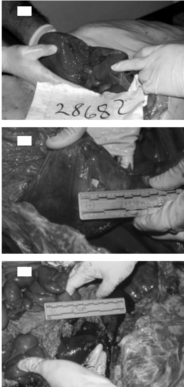
FIGURE 13. Typical injuries from free-back rigid-bar tests: (a) Liver laceration (CAD 28682/GI3); (b) Torn diaphragm (CAD 28838/GI6); (c) Splenic tear (CAD 29084/GI10).
