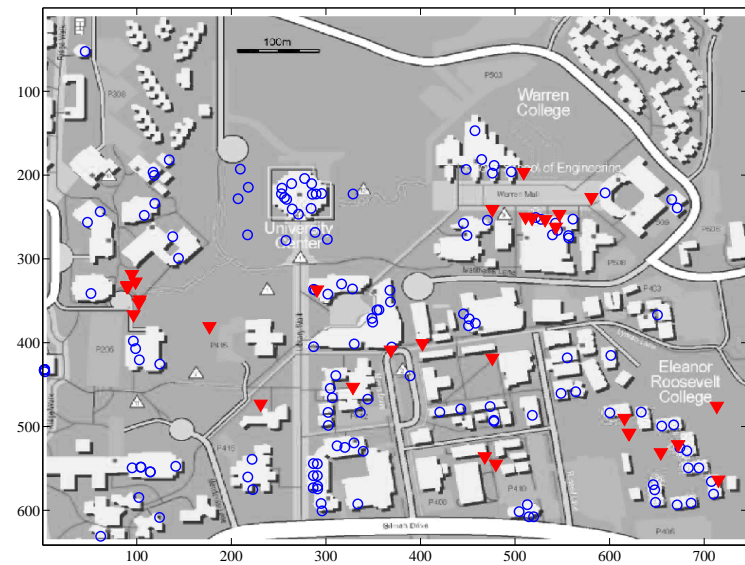
Figure 6.25: Location estimates of the unknown APs are shown in red. The known AP locations are shown in blue.
