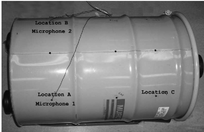
Fig. 8. Top view of the acoustic drum with two end-mounted actuating speakers, one disturbance speaker, and two internal microphones. Microphone 1 is initially at location A and is moved to location C, while the HSS control algorithm is operating. Microphone 2 is placed at location B throughout the experiment.
