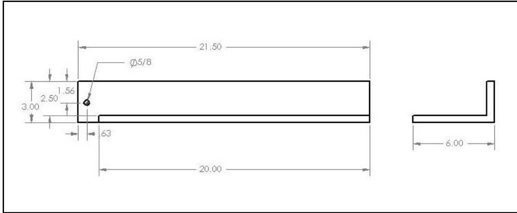
Figure D12. Dimensioned Drawing of L-shaped Motion Guide
