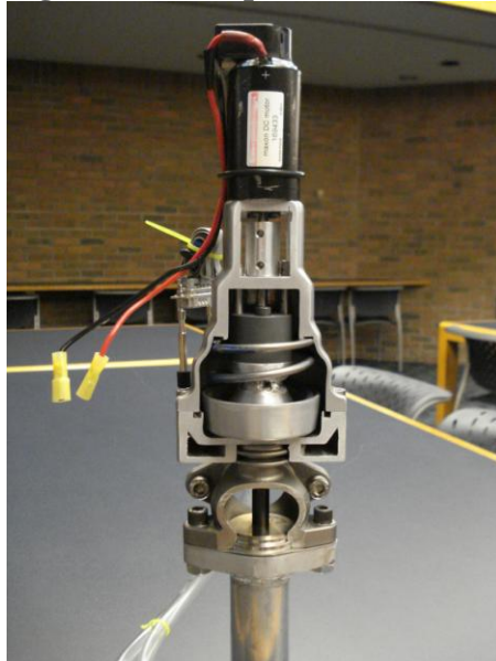
Figure 22: Completed Motor Control Exhaust Bypass Valve Prototype
