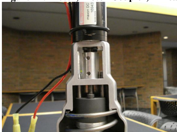
Figure 24: Motor, Motor Coupler, Threaded Rod Connection
