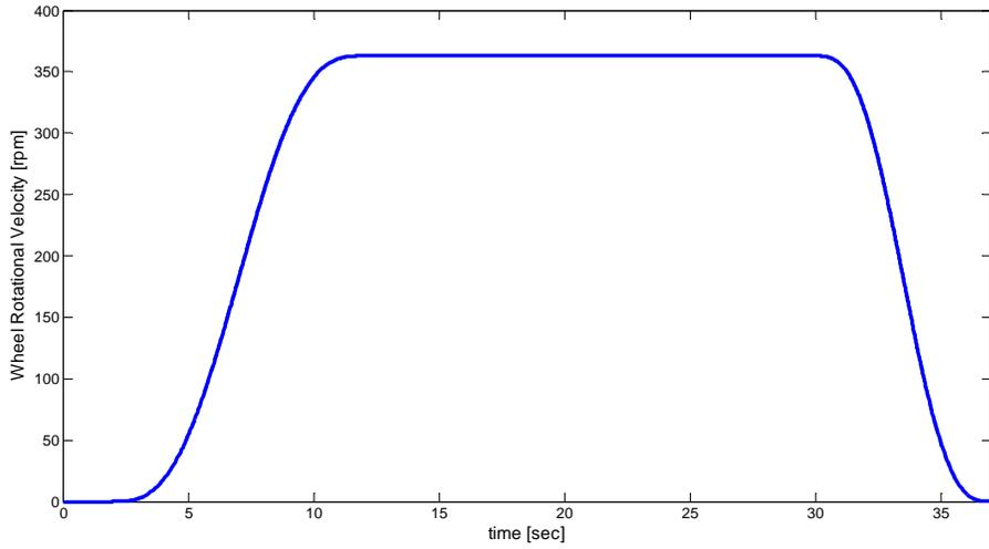
Figure 5.2: Wheel Rotational Velocity Input Profile
