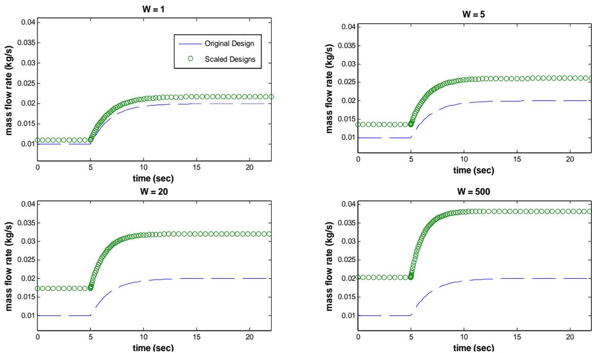
Figure 4.5: Mass flow rates of optimal scaled designs (fixed blower size)
