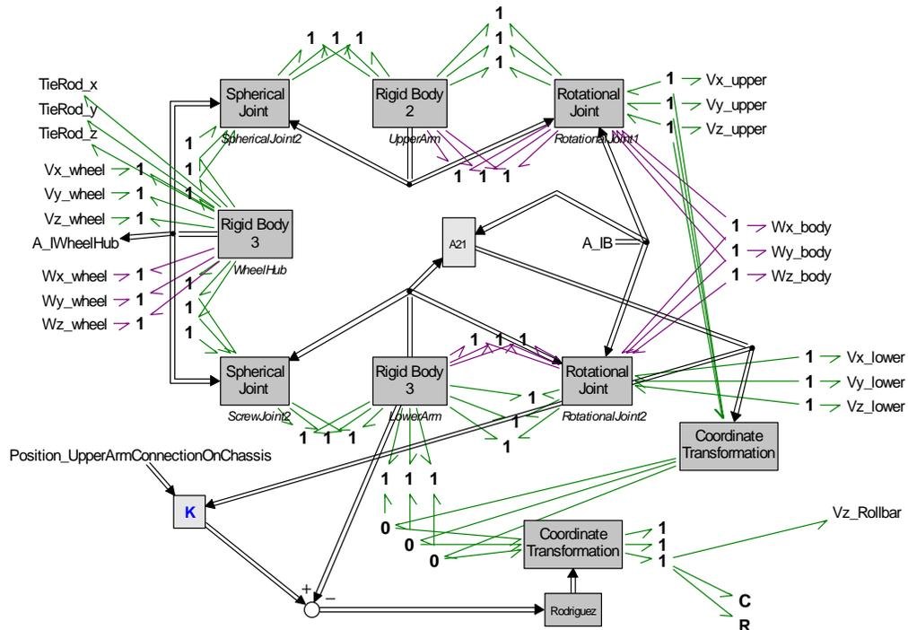
Figure E.2: Front suspension sub-model
