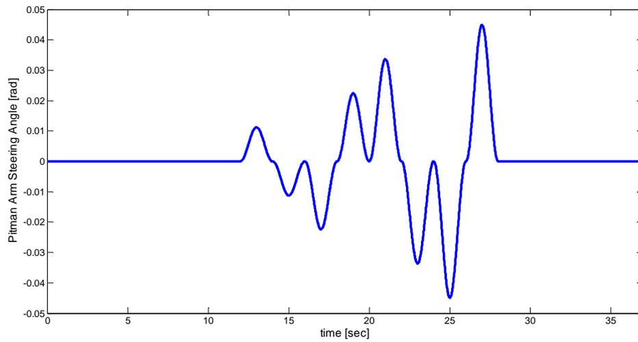
Figure 5.3: Pitman Arm Steering Angle Input
