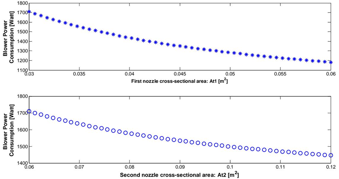
Figure C.2: Monotonicity in blower power consumption with respect to  $A_{t,1}$  and  $A_{t,2}$
