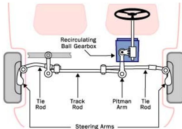
Figure E.8: HMMWV steering system components
