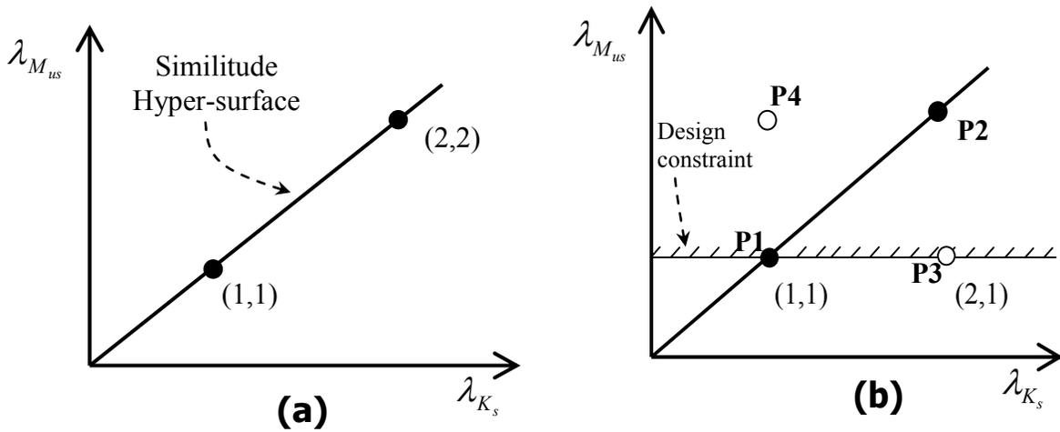
Figure 4.1: Scaling law coordinate system: (a) unconstrained, (b) constrained
