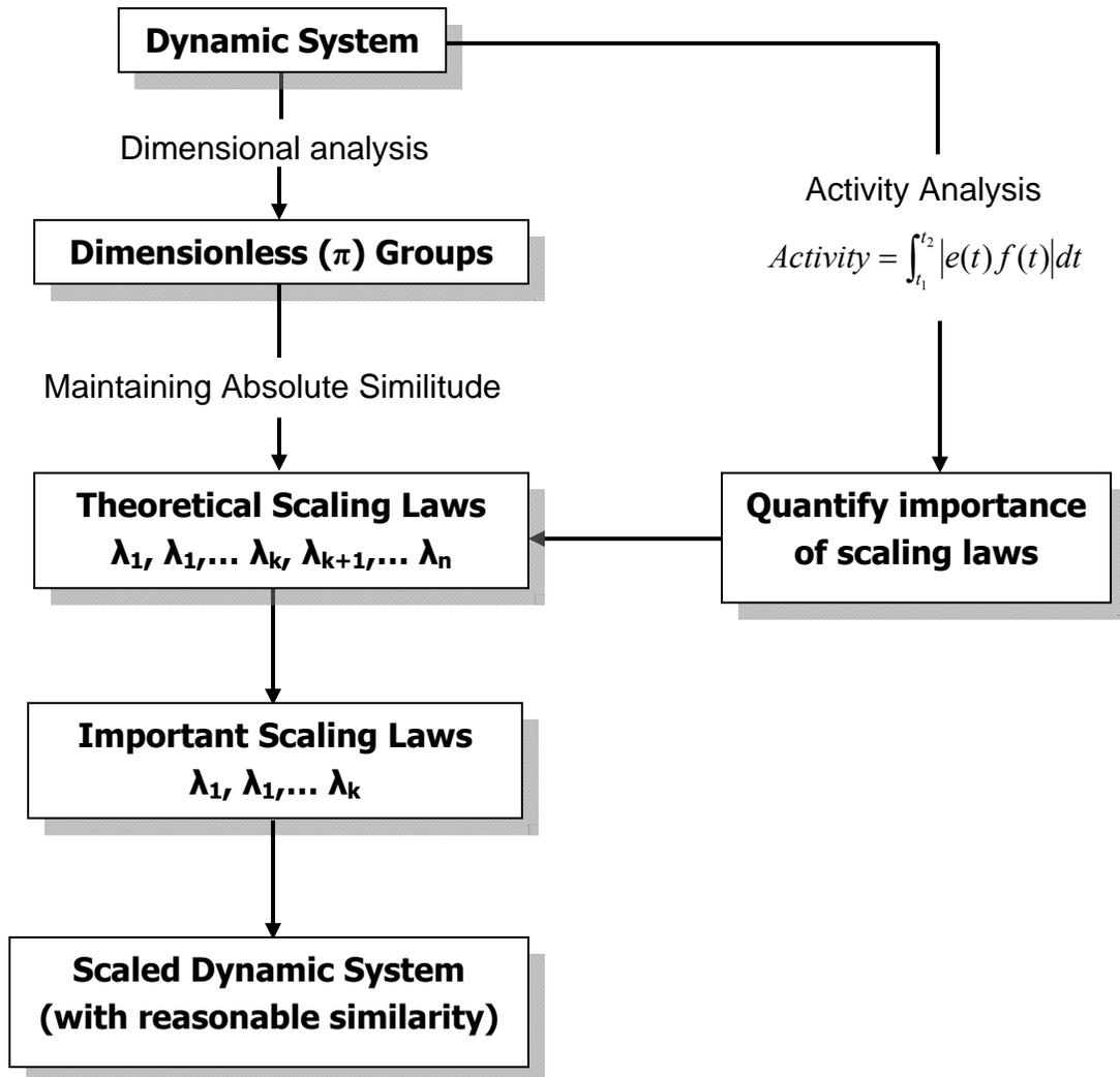
Figure 3.3: Scaling Methodology Using Dimensional and Activity Analyses
