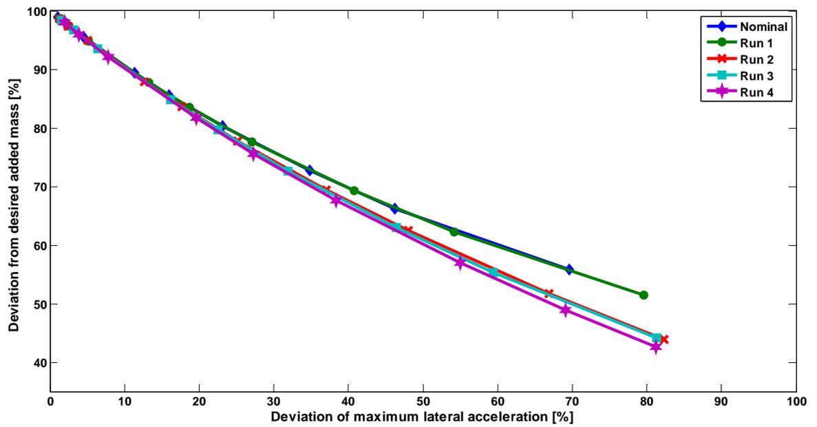
Figure 5.6: Trade-off between maximum lateral acceleration and added mass
