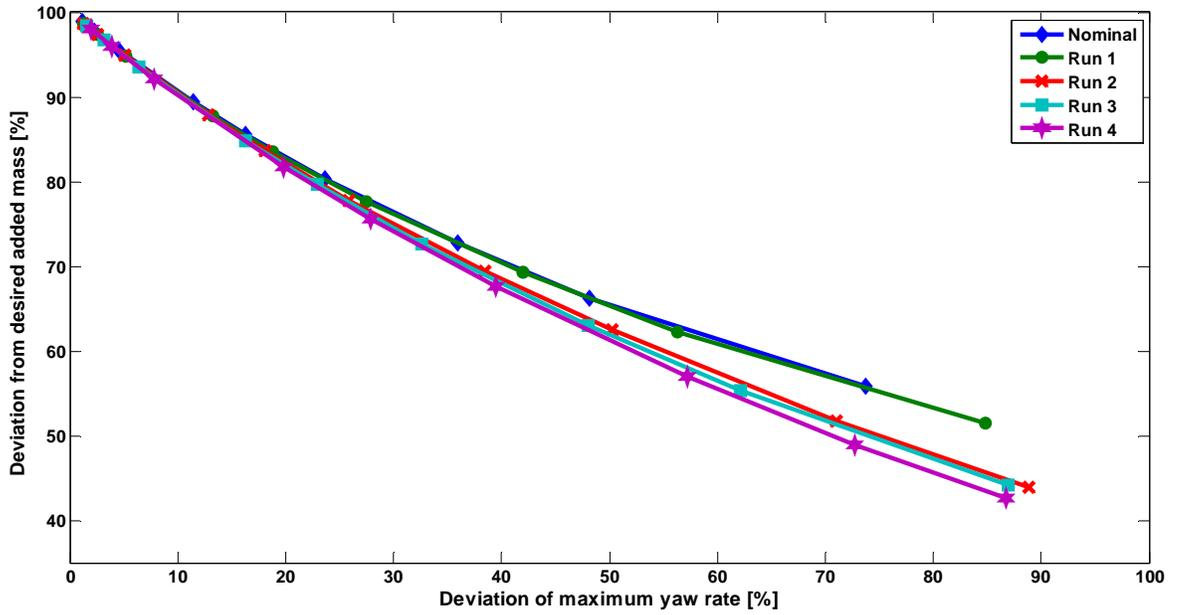
Figure 5.5: Trade-off between maximum yaw rate and added mass
