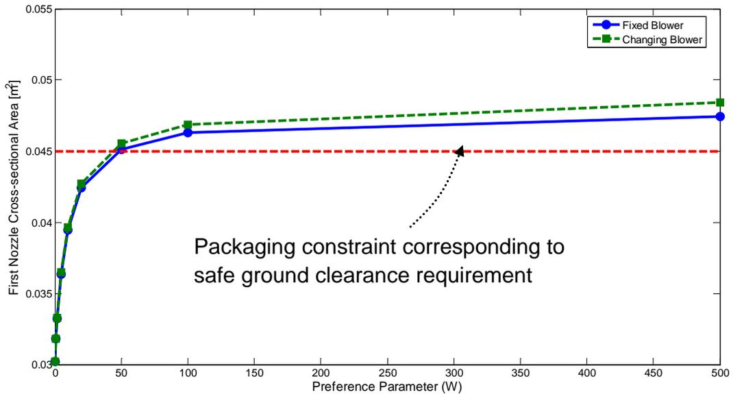
Figure 4.7: Influence of packaging constraints on scaling feasibility
