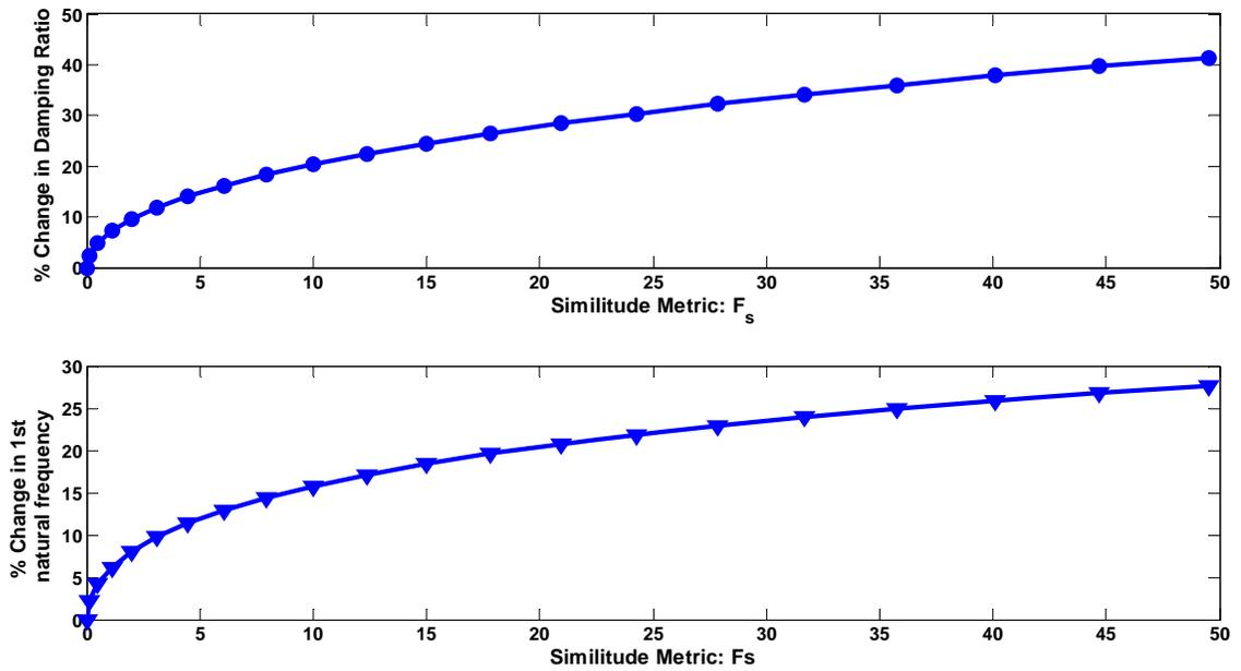
Figure D.1: Correlations between  $F_s$  vs. Damping Ratio and  $F_s$  vs. First Natural Frequency
