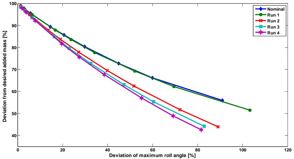
Figure 5.4: Trade-off between maximum roll angle and added mass
