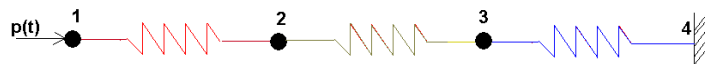
Figure 6.8: A one-dimensional model of fixed end cellular bar with three lumped masses
