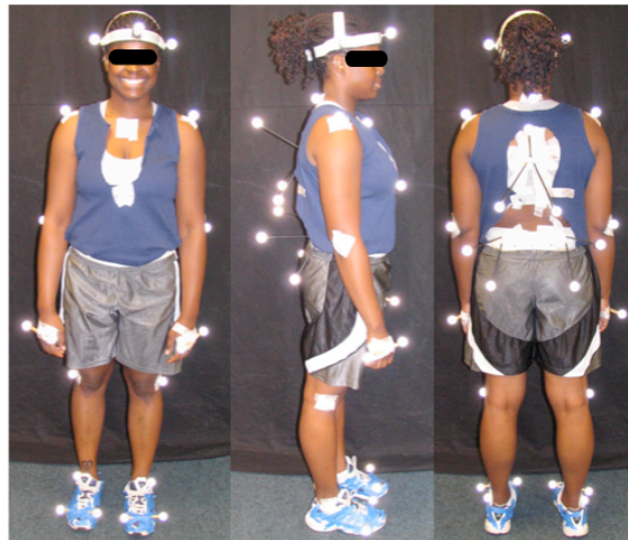
Figure 2.4. Retro-reflective marker set used to track whole-body motion.
