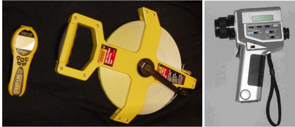
Figure 32. A 300 ft fiber glass tape and a 50 ft sonic laser tape to measure distance, and a recently calibrated Minolta LS-100 luminance meter to measure the brightness
