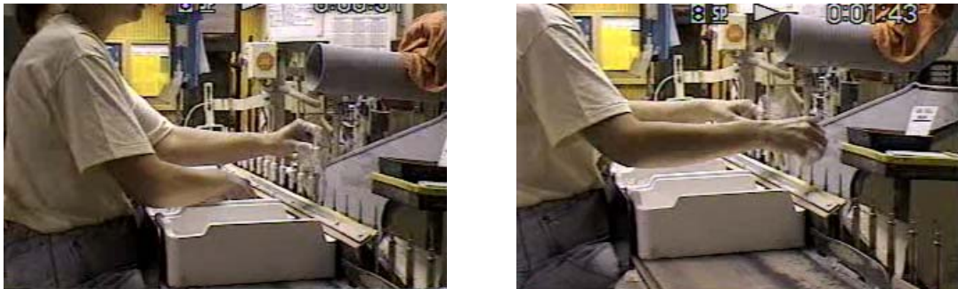
Figure 6.5 Insulator placement job. The worker grasped the insulators and put them on the pins moving in lateral direction
