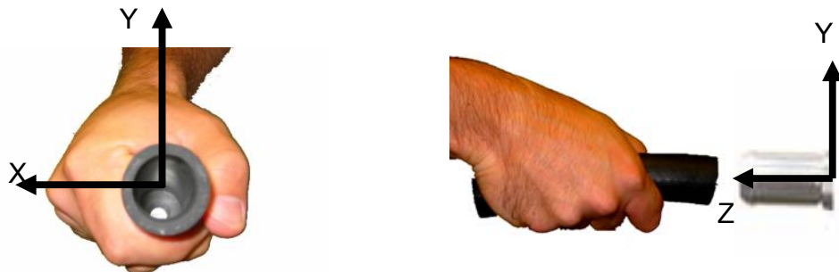
Figure 3.2 Definition of the new local coordinate system attached on the flange. The origin of this system is the center of the flange in the plane of the front end. Its x-axis is the unit vector to dorsal direction, its y-axis is the unit vector to superior direction, and its z-axis is the unit vector to the body.
