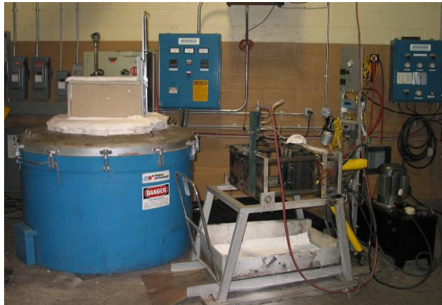
Figure 3.7 Permanent mold casting cell, ELM casting laboratories, Ann Arbor, MI.
