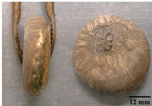
Figure 3.3 Button specimen cast after solidification analysis for microstructural investigations.
