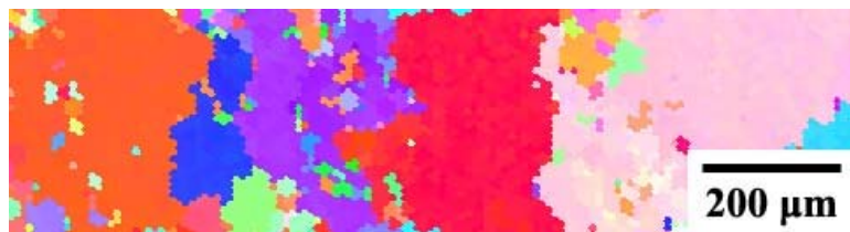
Figure 4.26 Orientation Image Map of AXJ530 for a region of the specimen gage.
