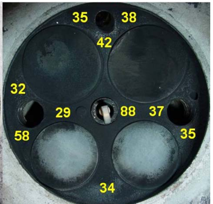
Figure 5.14 – CCD layer thickness on piston and head surfaces measured at the end of passive and aggressive conditioning
