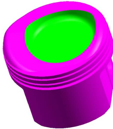
Figure 2.1 - Unigraphics model of GM MD-4 piston
