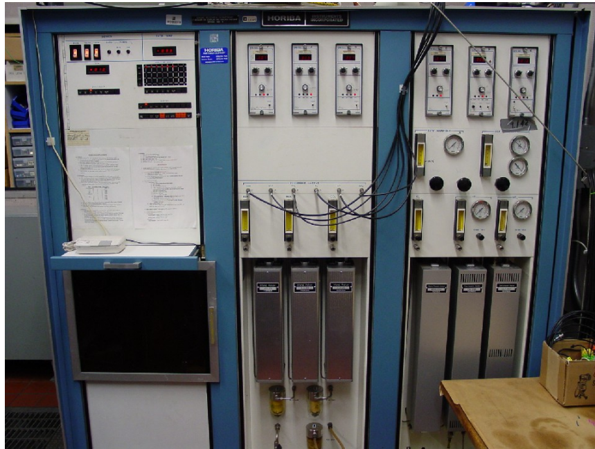
Figure 2.6 – Horriba emissions bench used throughout testing for analysis of engine out emissions and determination of operating air/fuel ratio
