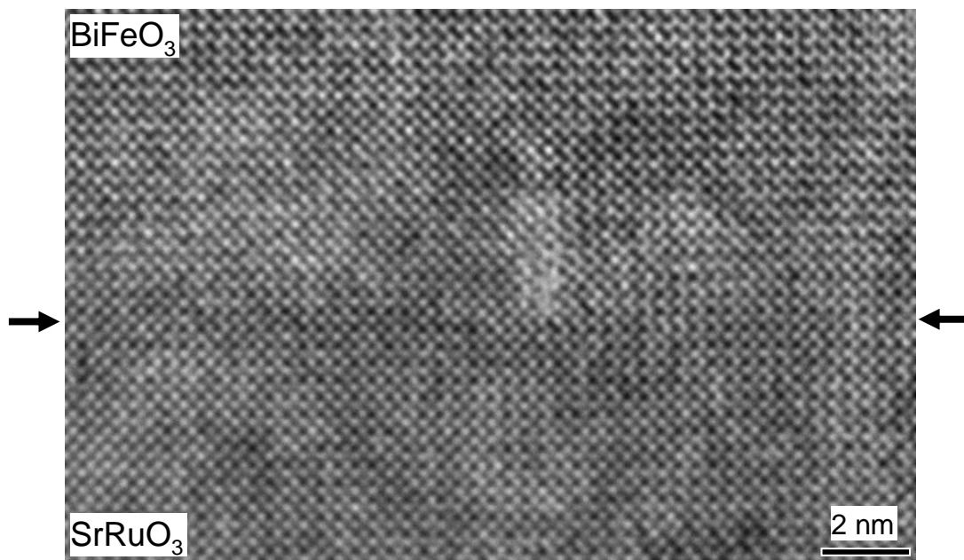
Fig. 3.11 The atomic structure of a misfit dislocation at BiFeO 3 /SrRuO 3 interface in sample 200 nm BiFeO 3 grown on 4° miscut SrTiO 3 substrate with 100 nm SrRuO 3 electrode.
