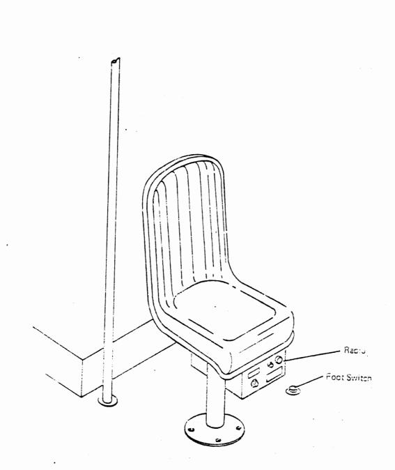
Figure 3 - Floorboard Switch for Silent Alarm
