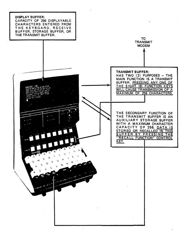
FIGURE IV. TRANSMIT BUFFER
