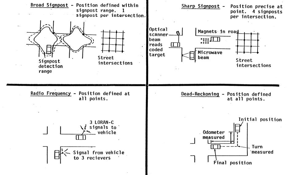
Figure 5 - AVM Location Subsystem Technologies
