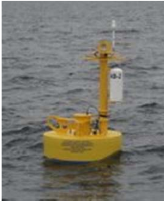
Figure 2. A real time auto detection buoy deployed in Cape Cod Bay. (NRWBUEOYS 2008).
