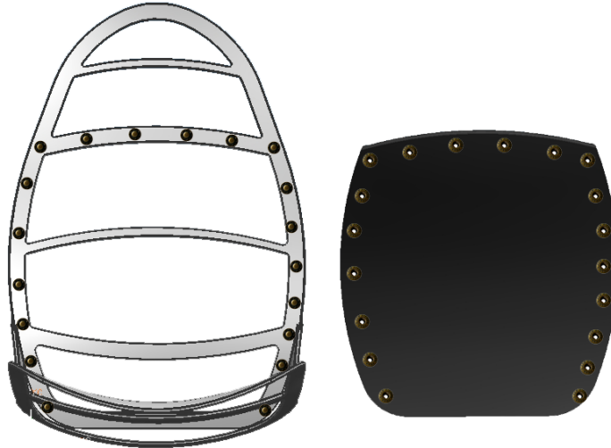
Figure 16: The cushion is attached with snaps for easy separation
