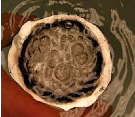
Figure 30. Gas diffusion across porous ceramic gas diffuser
