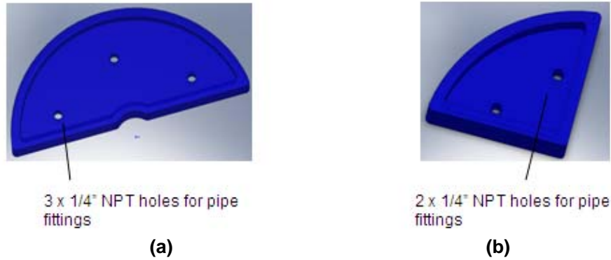
Figure 18. Top view of (a) Half showerhead part and (b) Quarter showerhead part
