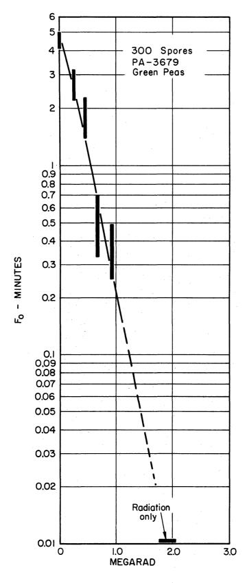
$F_{\rm O}$  required to sterilize green peas packed in No. 1 Picnic tin cans, inoculated with 300 PA-3679 spores per can, and irradiated with gamma rays from Cobalt-60 before heat processing at 230°F and incubation at 85°F.
