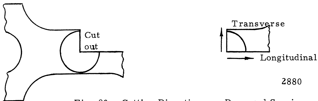
Fig. 83. Cutting Directions on Damaged Specimen.
