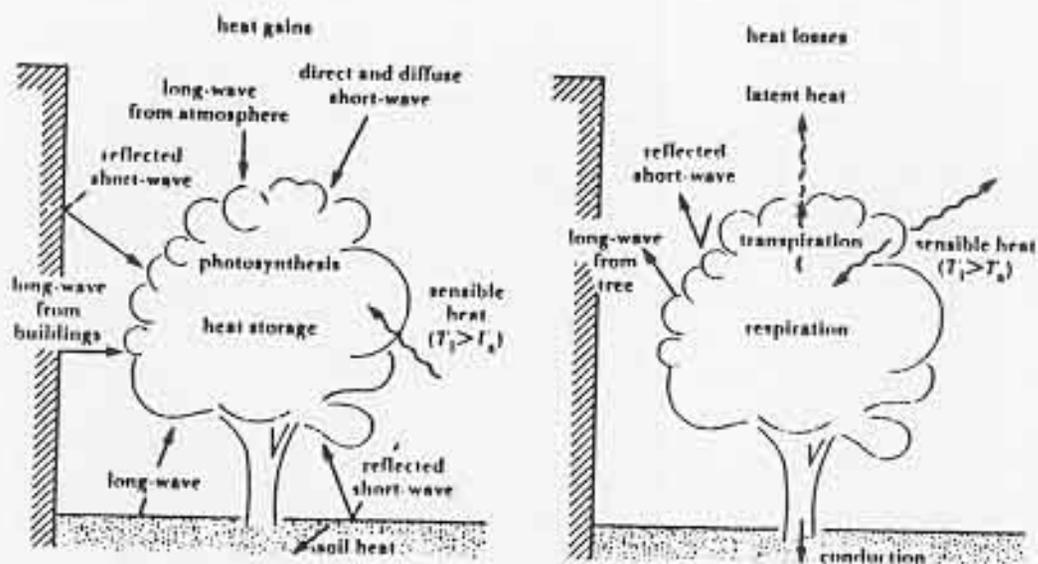
Fig. 1 Energy Balance of an Isolated Tree
