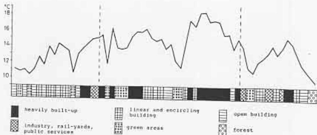
Fig. 5 Air Temperature Traverse @ 2m Above Ground
