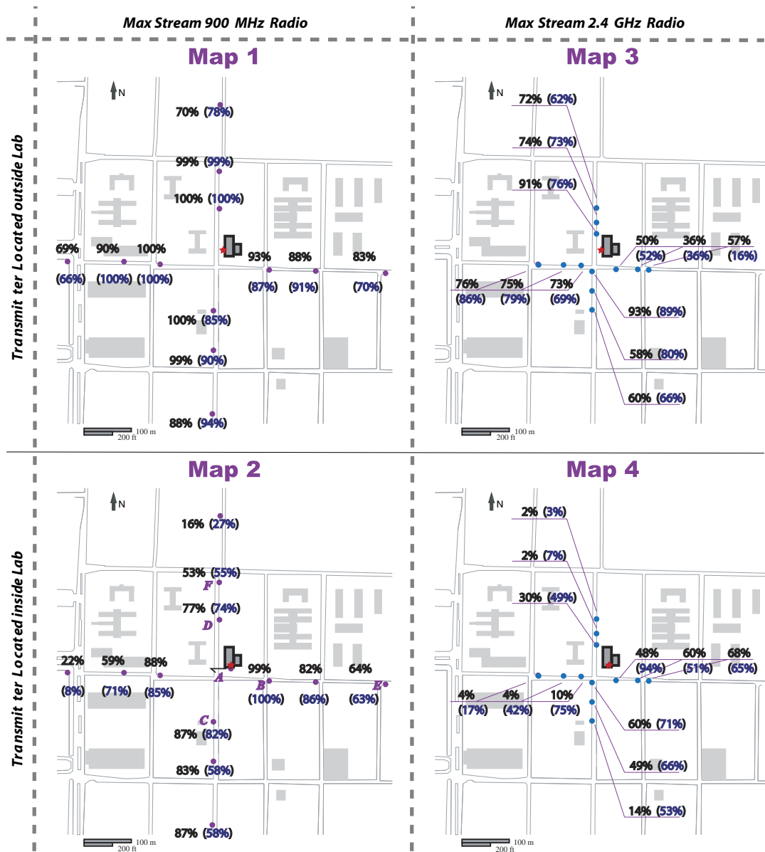
Figure 5. Results of loopback tests of MaxStream 9XStream radio (900 MHz) (in Maps 1 and 2 at the left column) and 24XStream radio (2.4 GHz) (in Maps 3 and 4 at the right column). The values without parentheses were recorded in fall, while the values inside parentheses were recorded in winter.
