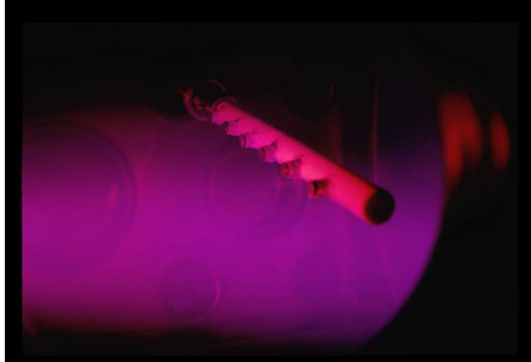
Figure C.10: Flux probe array inserted in the exhaust plume. Multiple planar collectors are spaced along an alumina ceramic tube.
