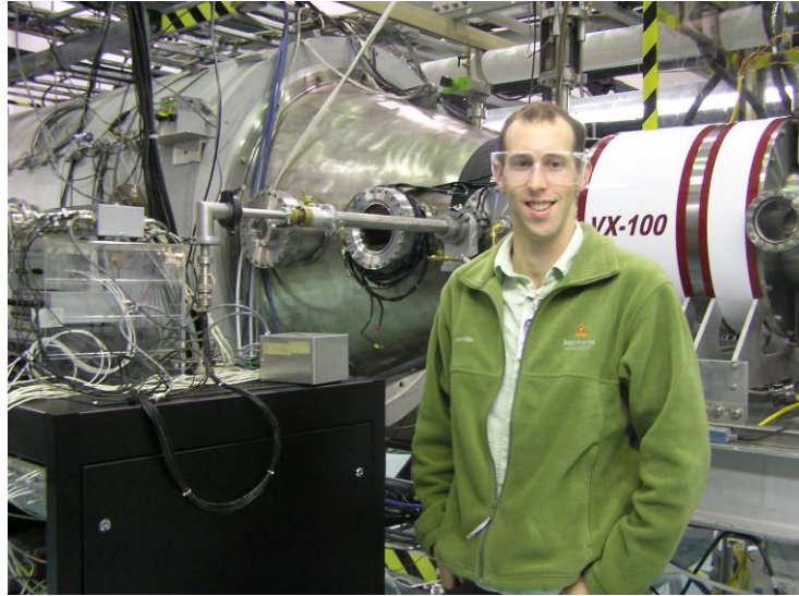
Figure C.1: The author in front of the VX-100 laboratory experiment. The left side of the picture shows the 4 m 3 vacuum dump tank connected to the conical expansion section. Electrical feedthroughs and viewports allow access to the plasma in this expansion section.
