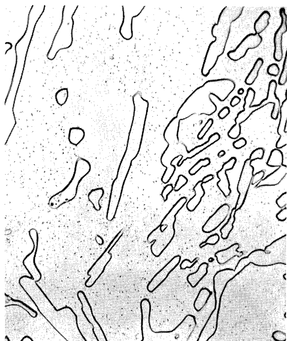
D. R309, 1.49% B, Austenite Hardness, 129 kg/mm 2 .
