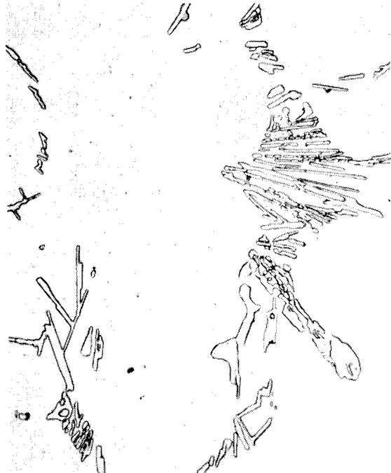
1926-01 B. R312, 0.32% B, 9.92% Boride By Volume. Austenite Hardness, 139.5 kg/mm 2 .
