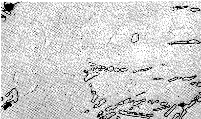
2323-01 B. R344-7, 0.50% B Aim Analysis. 8500 psi Load, 382-hr. Life.
