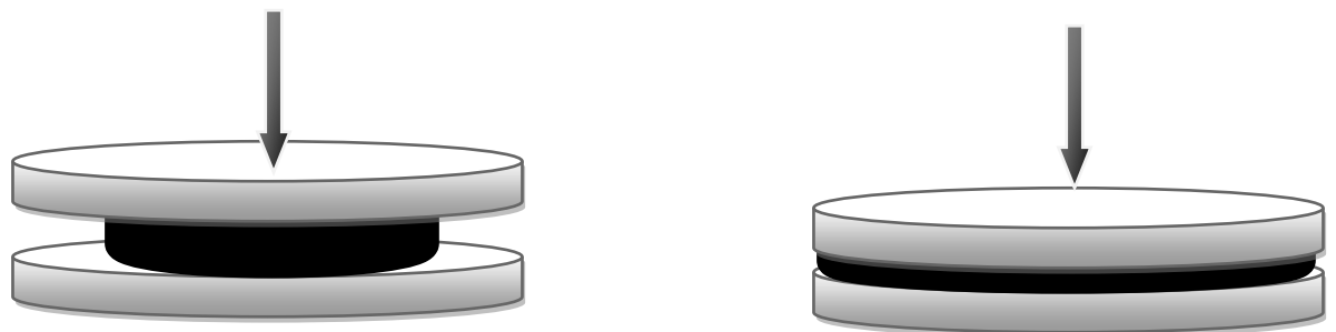
Figure 1.1 Constant Volume Squeeze Flow with black mass compressed between plates
