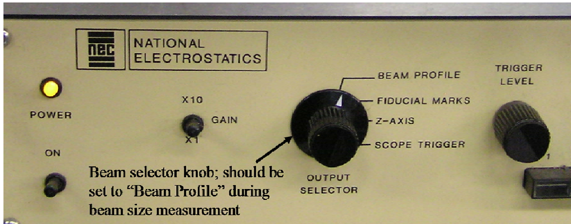
Figure 4.13 Beam profile monitor, including the beam selector knob set at 'beam profile' for beam size measurements.
