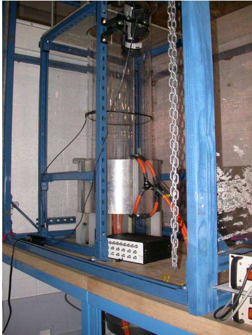
Figure 2.10: Photograph of the annular chamber, test setup, and current transmission cables
