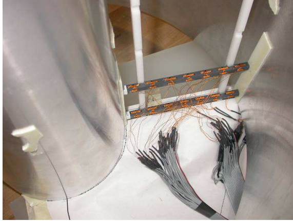
Figure 2.22: 3-axis internal field probe setup testing coil discharge uniformity
