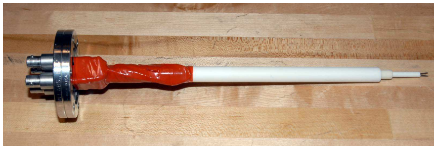
Figure 2.44: Photograph of the triple probe used for the XOCOT discharge experiment
