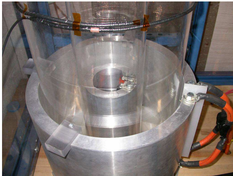
Figure 2.11: Annular Discharge Coil used in the discharge experiment
