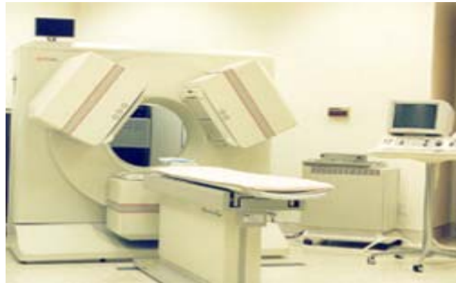
Figure 1.2 A commercial SPECT system with triple imaging heads at 60 degrees to each other. (Picker PRISM 3000). This system can have three times the sensitivity as the single head system in Figure 1.1 and also rotates around the patient to obtain full angular sampling.
