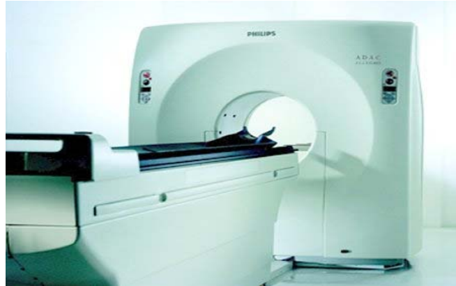
Figure 1.3 A PET system. (Philips Allegro). The detector forms a ring around the patient to obtain full angular sampling and detects the annihilation gamma ray pairs in coincidence.
