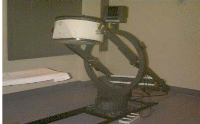
Figure 1.1 A planar collimated Anger gamma camera for detecting \gamma -ray photons from the radiotracer in whole body imaging.
