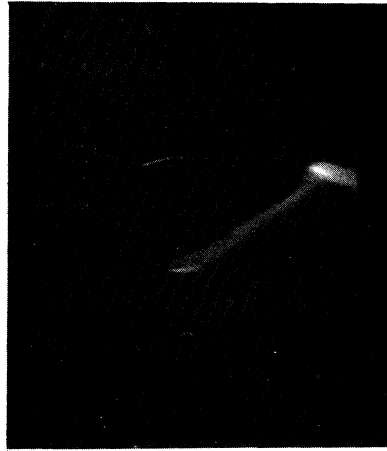
Fig. 2. Polaroid photograph of arc reflection in side-wall of tunnel. M_{\infty} = 2.5 , P_t = 12.9 in. Hg, I = 425 amp, gap = 1.1 in.
