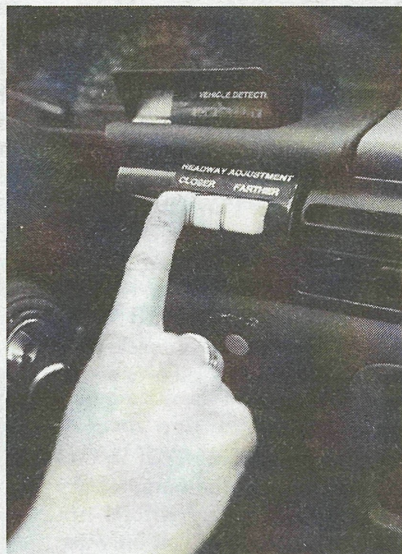
The author changes a setting that controls the distance between her vehicle and the one ahead.
