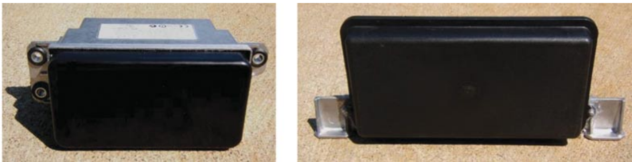
Figure 7. Delphi radars: 76-GHz ACC (left) and 24-GHz BUA (right).
