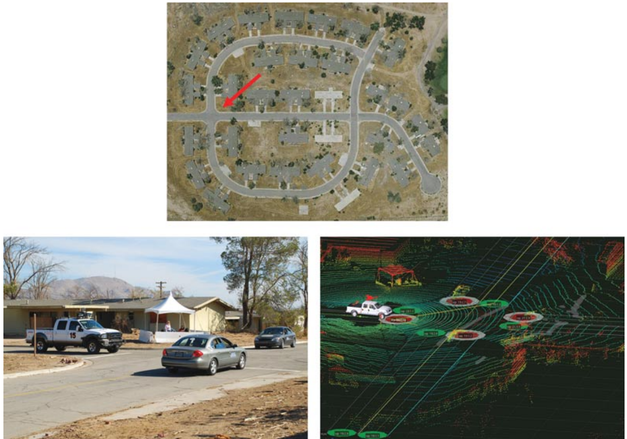
Figure 22. Area C: intersection logic and dynamic replanning. Aerial photo of Area C course (top); red arrow indicates the intersection depicted in the figures below. XAV-250 successfully exhibits advanced traffic behavior (bottom left). MIT viewer rendering of the RNDF and tracked cars at the intersection (bottom right).
