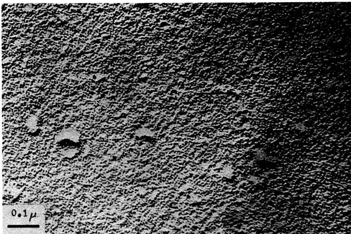
Figure 56: Atactic polystyrene M_w=1,800,000 stretched 100% on mylar. Platinum shadowed at 30^\circ . Stretch direction is horizontal.
