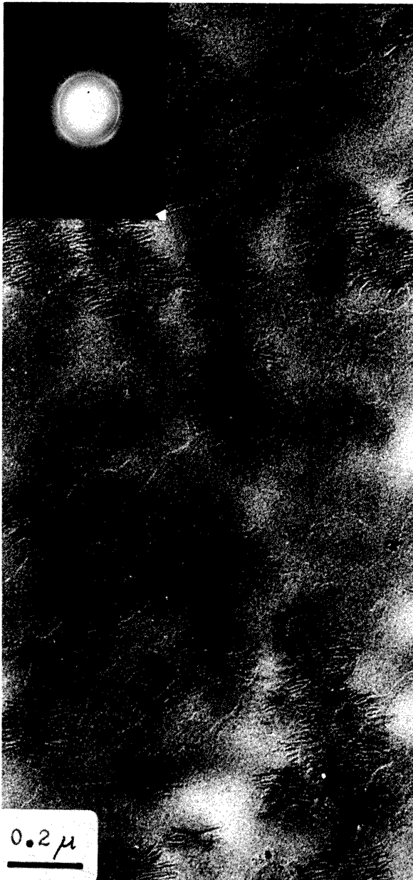
Figure 43: IPS/benzophenone 60/40 stretched 300%, annealed at 125°C for 6 minutes. Platinum shadowed at 30°.
