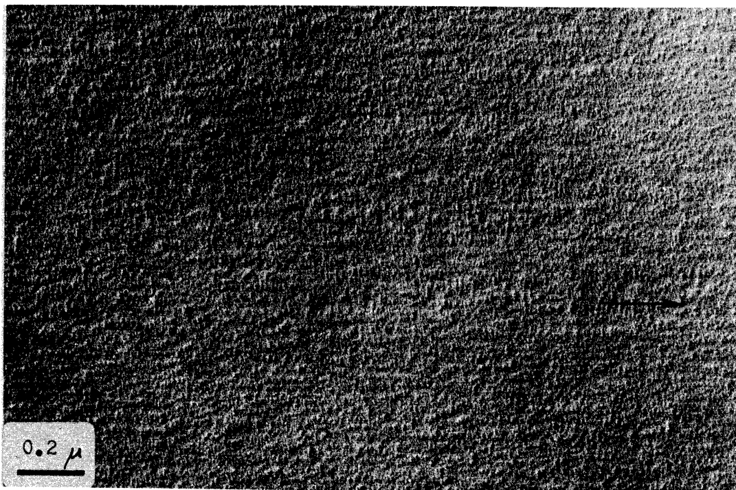
Figure 53: Isotactic polystyrene/benzophenone 60/40 stretched 500%, annealed at 155°C for 6 minutes. Platinum shadowed at 30°. Stretch direction is horizontal.
