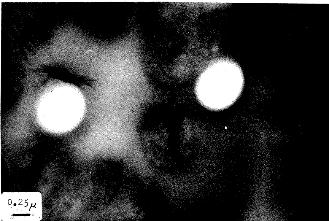
Figure 26: Isotactic polystyrene holey film crystallized on glass slide at 140°C for 10 minutes. Gold decorated at 90°.
