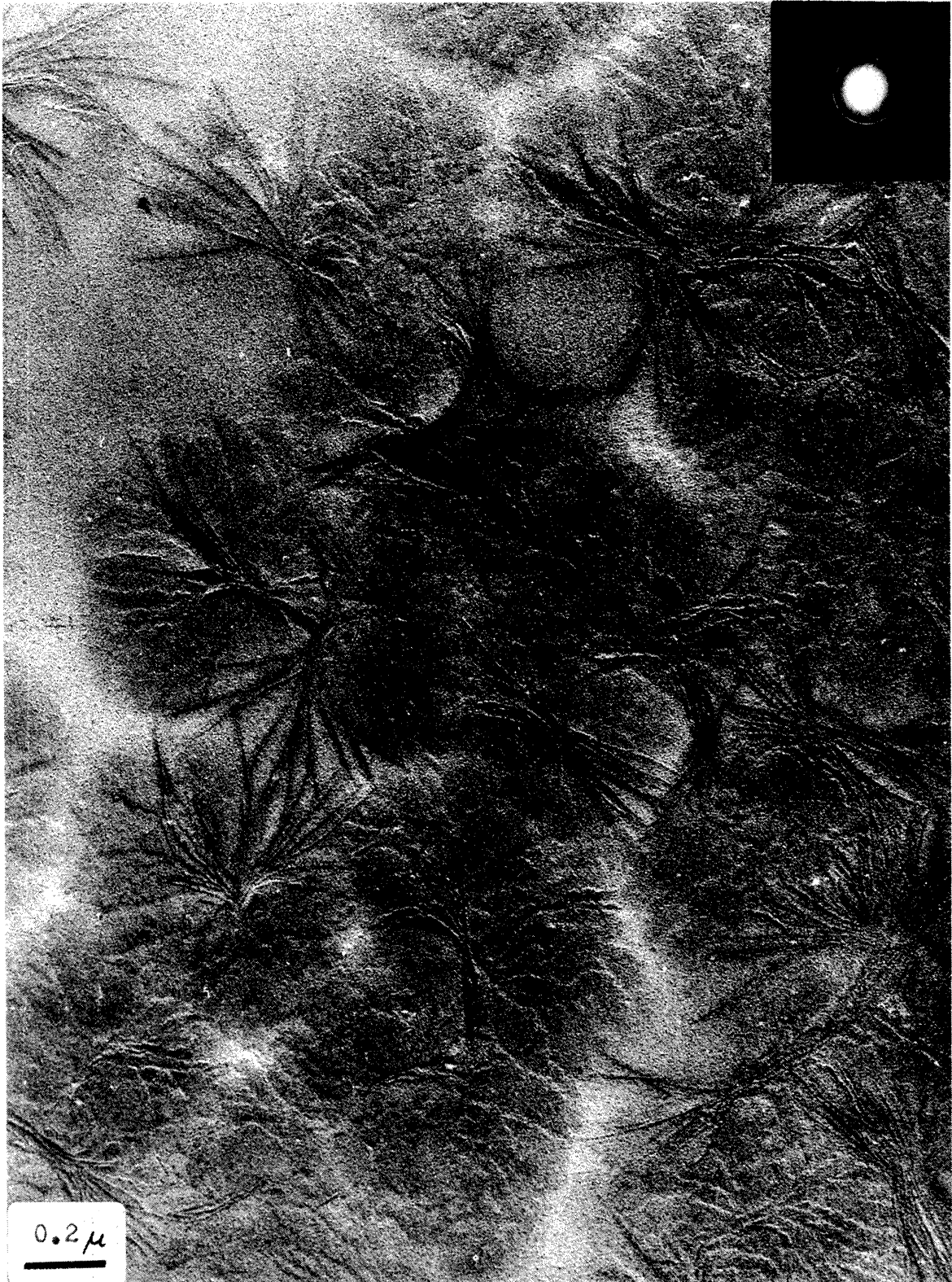
Figure 3: Electron micrograph of isotactic polystyrene crystallized from the glassy amorphous state at 140°C. Platinum shadowed at 30°.
