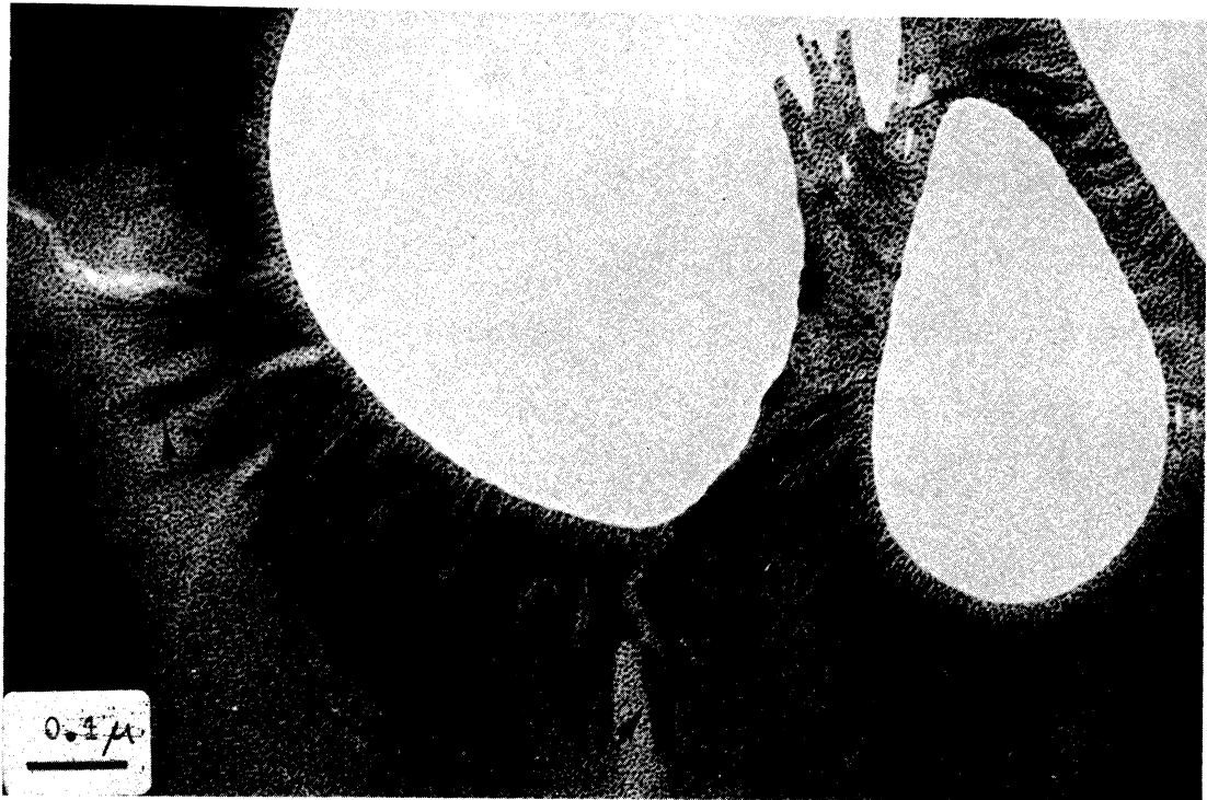
Figure 31: Isotactic polystyrene holey film crystallized at 140^{\circ}\text{C} for 10 minutes. Gold decorated at 90^{\circ} . Dense crystalline regions are indicated by arrows.
