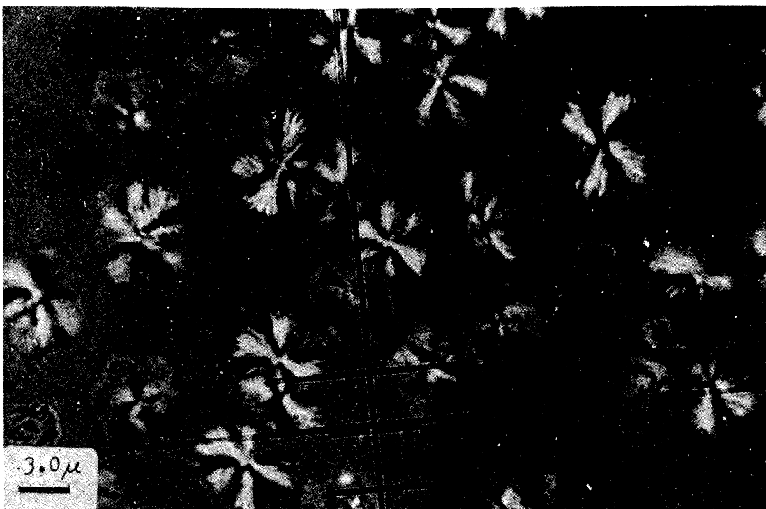
Figure 4: Light micrograph (through crossed polarizers) of isotactic/atactic polystyrene 40/60 (APS M_w=19,800 ) crystallized from the melt at 180°C. Arrows indicate serrated edge of spherulite.
