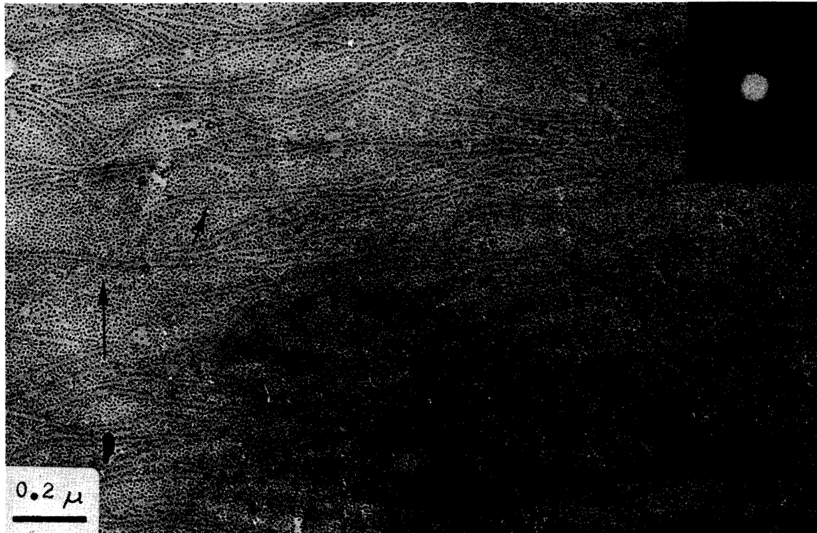
Figure 34: Isotactic polystyrene stretched 100% on mylar, annealed at 175°C for 5 minutes. Gold decorated. Stretch direction is vertical. Small arrows indicate tri-layer decorative pattern.
