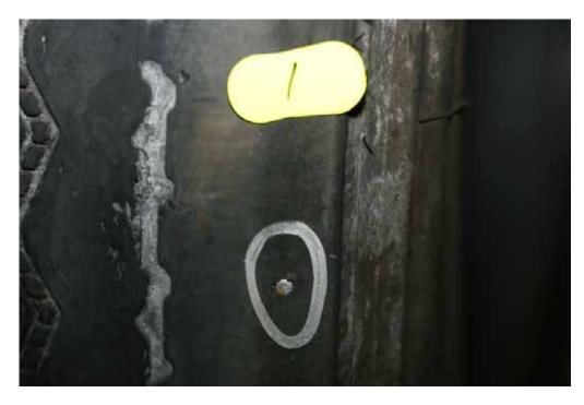
**Figure 9.2 - Overdeflected Operation #1** - Apparent nail in outer rib, resulting in slow air loss and flex fatigue damage
