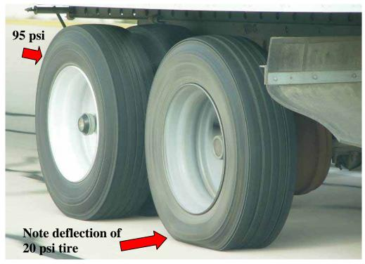
**Figure 5.5 – Underinflated Tire** Note: Tire Size 295/75R22.5, 5770 lbs, Speed 70 MPH and Load 5,770 pounds Courtesy Bridgestone/Firestone
