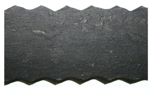
Figure 9.18 - Manufacturing/Process Issues #4 - Bond failure at buff line
