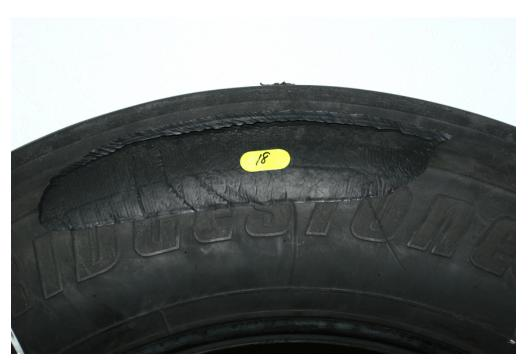
**Figure 9.13** – **Maintenance/Operational #2** - Use of improper (outside-in string plug) repair. Resulted in excessive intracarcass pressurization, sidewall separation, and tire failure
