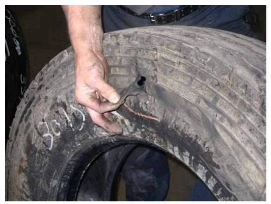
Figure 2.5 – Hands-On Inspection of Casing
