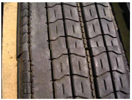
**Figure 5.4 – Misaligned Splice on a Pre-Cure Retread Casing** Source: O. Page
