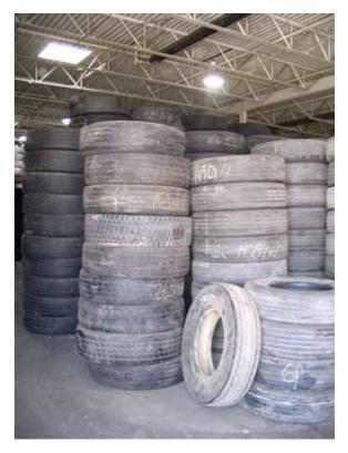
Figure 2.4 – Casings Received for Retreading
