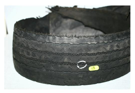
Figure 9.10 - Road Hazard #3 - Unrepaired crown puncture in original tread
