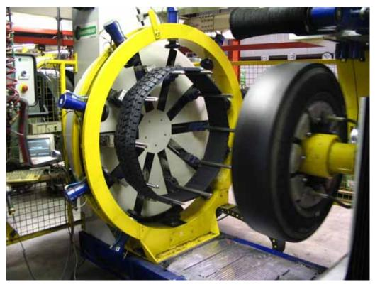
Figure 2.12 – Application of New Tread (Ringtread Process)
