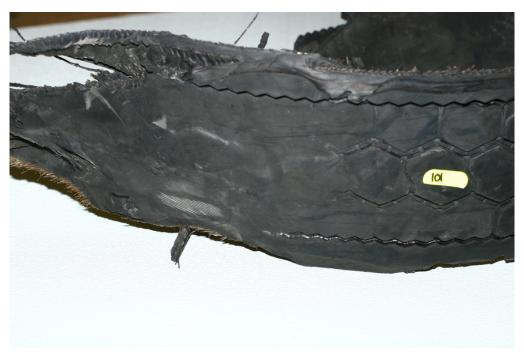
**Figure 9.14 – Maintenance/Operational #3** - Example of drive axle tire with localized accelerated wear
