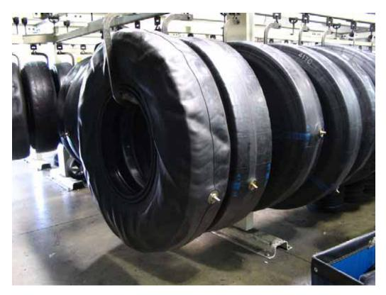
Figure 2.13 – Pre-Cured Retread Casings Enveloped
