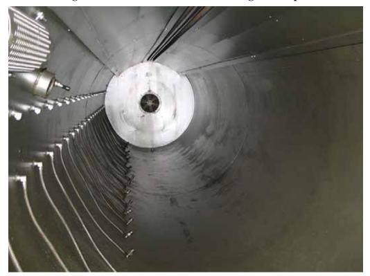
Figure 2.14 – Inside Vulcanization Chamber
