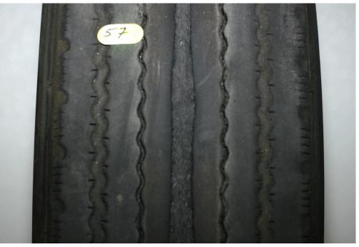
**Figure 9.15 - Manufacturing/Process Issues #1** - Retread rubber separated at buff line. This resulted in a "raised" section of the tire's circumference. Localized, accelerated wear (9" in the center of the tread) resulted, extending to the buff line.
