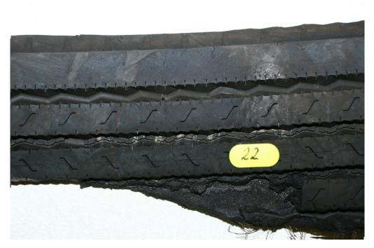
Figure 9.7: Excessive Heat #4
