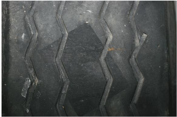
Figure 2.25 – Tread Pattern on a Regrooved Tire (Note: Amateurish Tread Pattern Design) Source: Smithers Scientific Service Inc.
