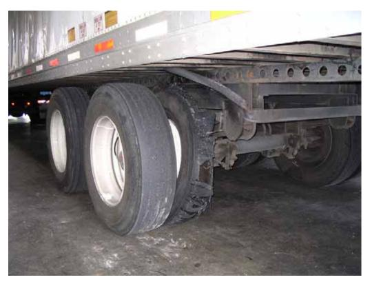
Figure 5.1 – A Failed Medium-Duty Truck Tire
