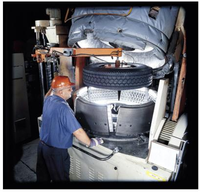
Figure 2.19 – Removing Casing from Retread Mold (Mold Cure Process) Courtesy of Bridgestone Firestone
