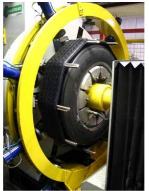
Figure 2.23 – Precured Tread (Unbroken) Brought Into Place around Casing (Ring-Tread Process)
