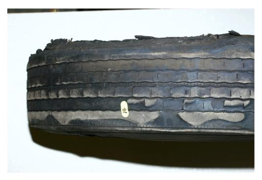
**Figure 9.4 - Excessive Heat #1** (This overdeflected tire showed vibrant bluish discoloration, characteristic of operating at excessive temperatures)
