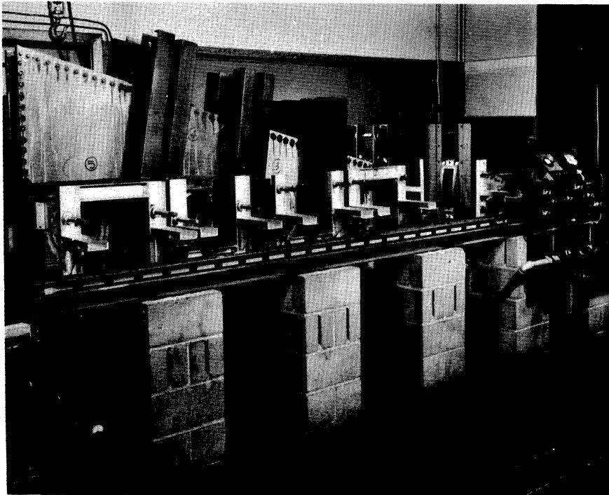
Fig. 4. The assembled sector shock tube with the vacuum and pressure control system.
