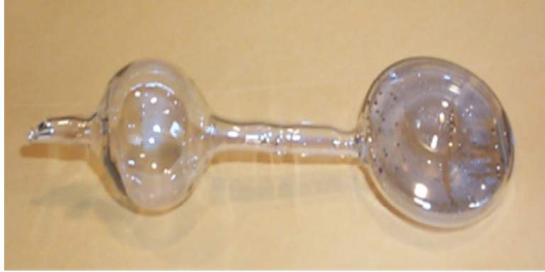
Figure 4.16: A double cell, “Tweety”. In double cells pumping is done at one part and this part is not exposed to neutron beam to avoid the depolarization due to ionization.
