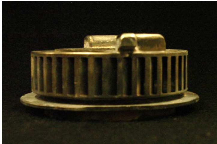
Figure 2.8: Photos of the swirl cup or mixer that generates the swirl for the main annulus.
