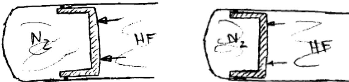
Figure 6 – A basic piston accumulator, with a single o-ring seal.
