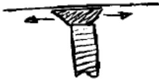
Figure 39 –Trapezoidal Dual-Scraper Seal.
