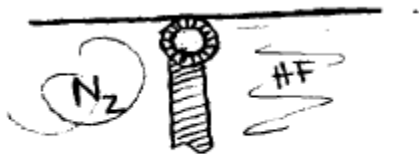
Figure 46 – Inflatable Seal System Design
