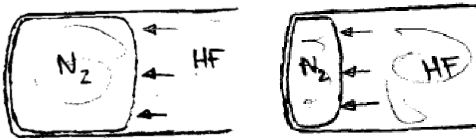
Figure 3 – Basic elastic bladder design, with nitrogen inside the bladder on the left and hydraulic fluid outside on the right.
