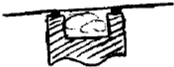
Figure 44 –Dual Seal System
