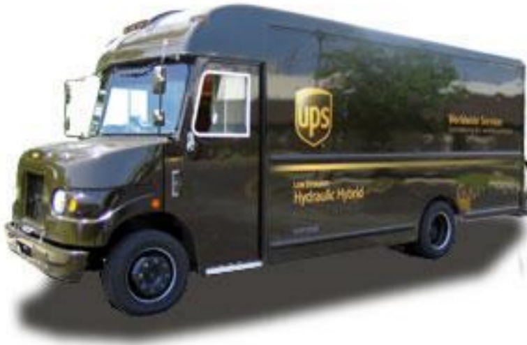
Figure 2 – Hydraulic Hybrid UPS truck created by the EPA [2]
