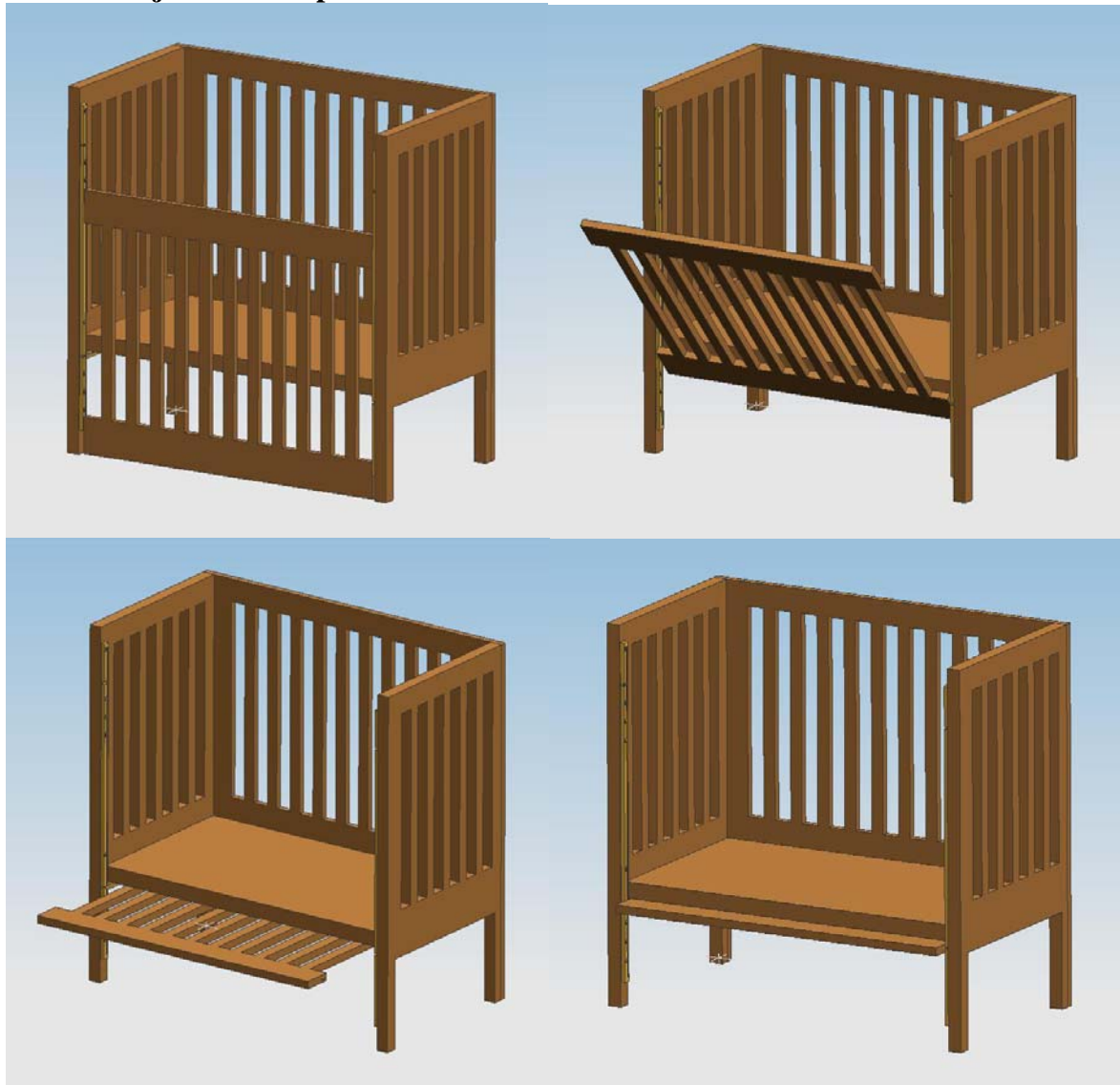
CAD-3: Adjustable Drop Side that can be stowed underneath the Mattress base
