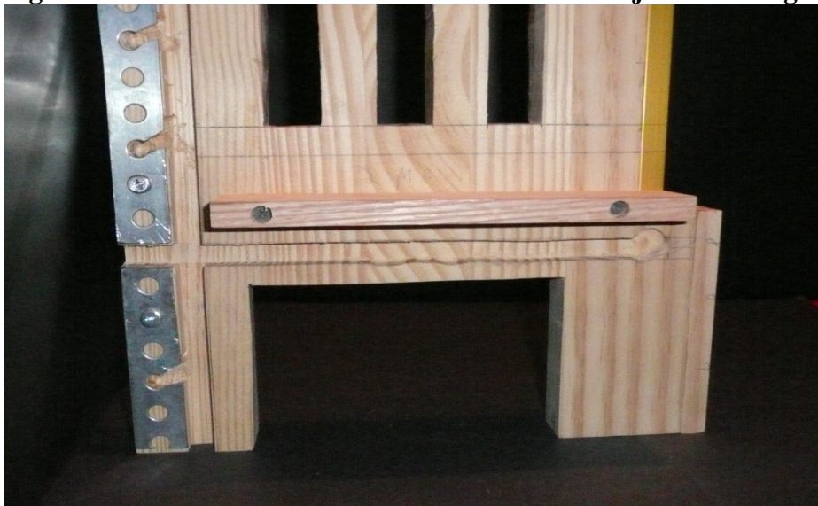
Figure-P4: Channels for Front Rail and Holes to Adjust The Height of the Front Rail
