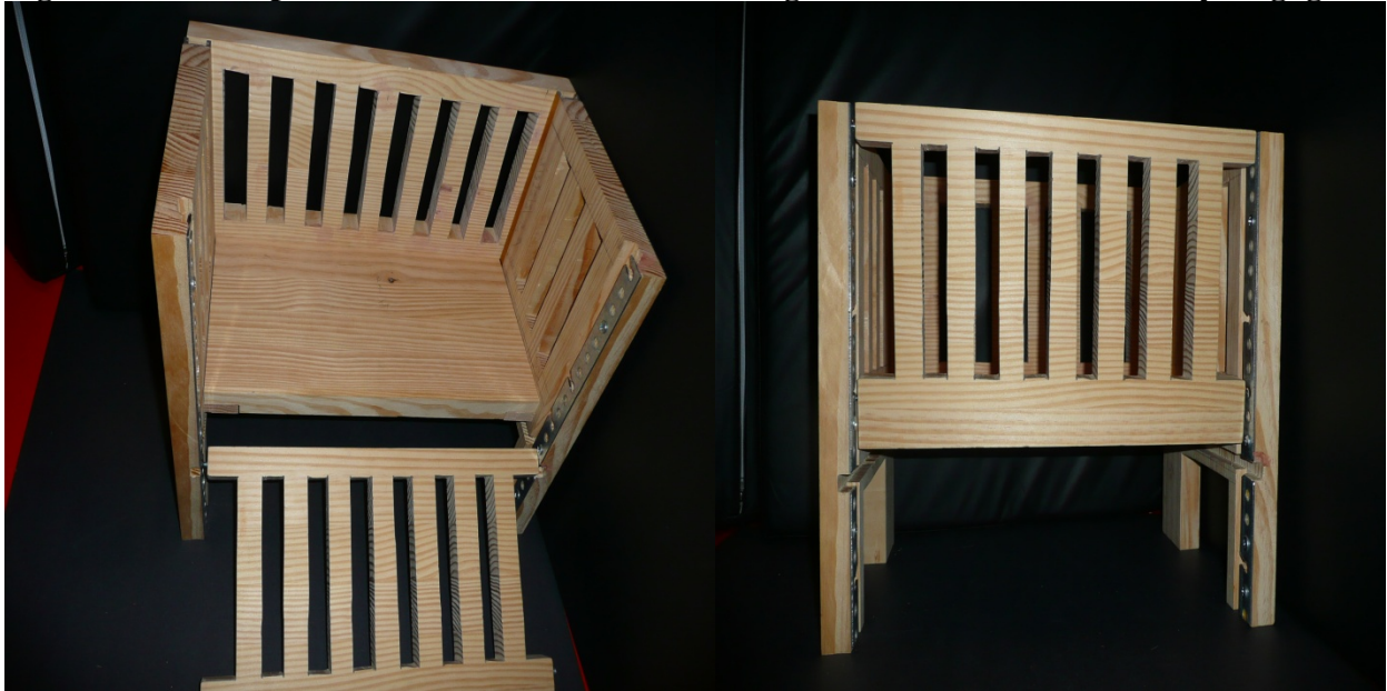
Figure-PAS5: Step-1 of Front Rail Installation Figure-PAS6: Front Rail Fully Engaged
