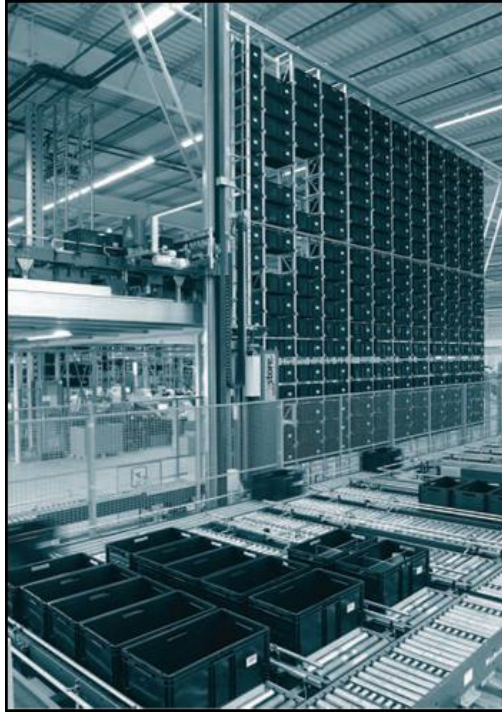
Figure 57: Viastore Systems' Viapal S/R application can retrieve and store containers
