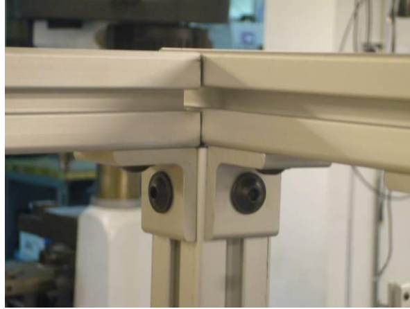
Figure 32: Corner interface of the system frame
