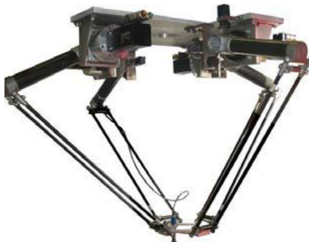
Figure 58: The Quickplacer robot processes parts at a rate of 215-250 parts per minute.
