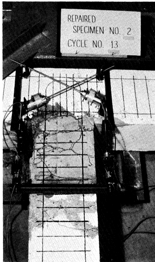
Fig. 5.1 Repaired Specimen 2 after Retest
