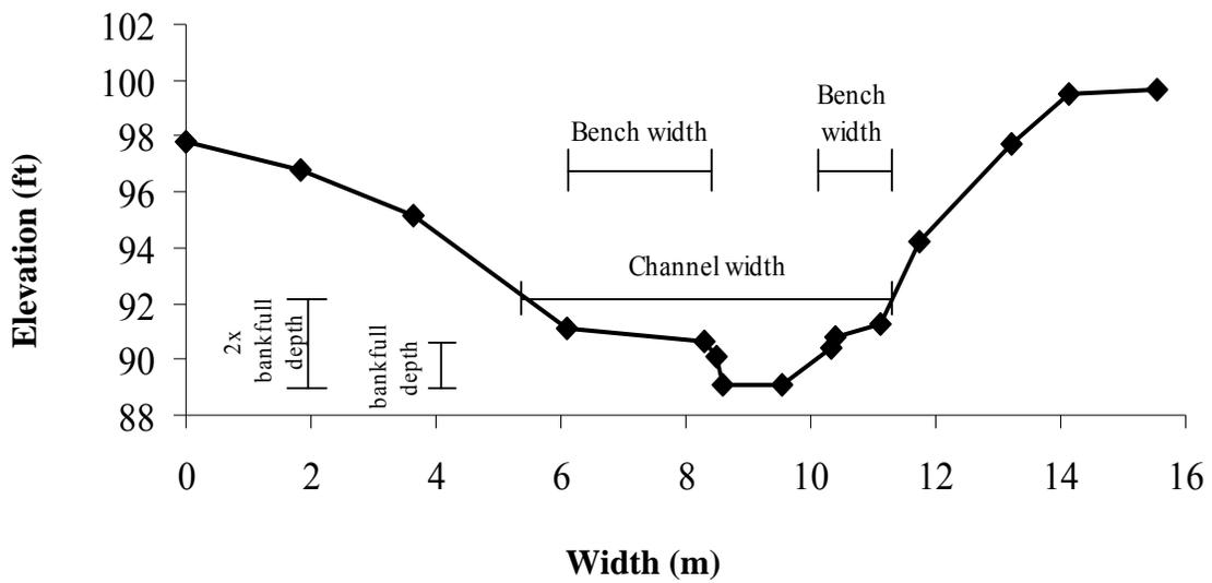
Figure 2. Cross-section depicting channel morphology measurements at the benched metabolism site (data courtesy of Janssen 2008).
