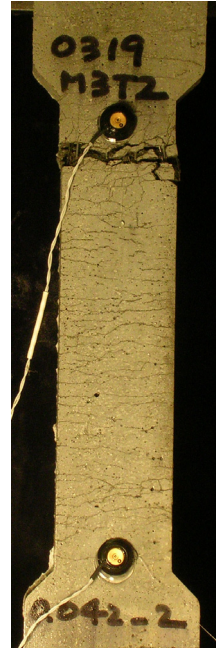
Fig. 3.6- Tensile stress – strain curve and cracking behaviour
