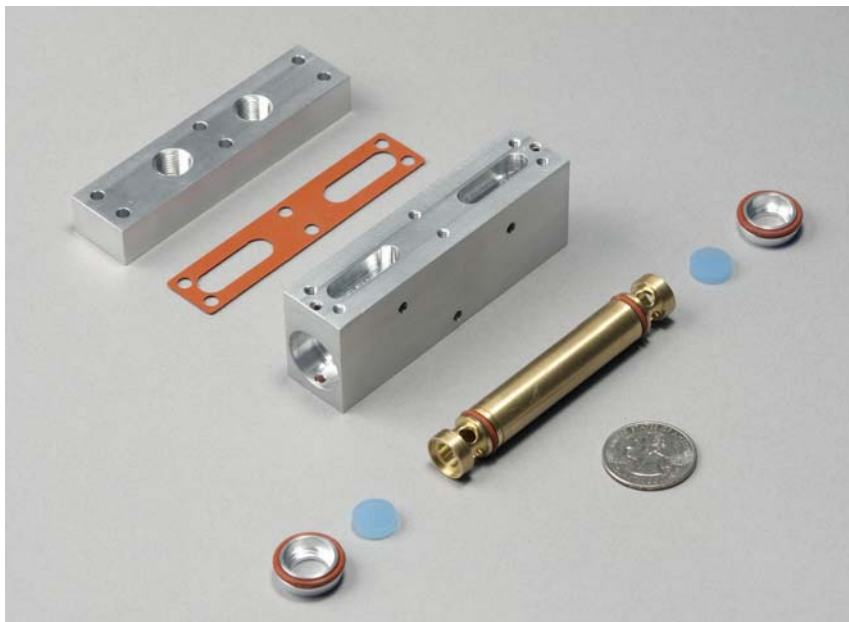
Figure 6.2. Components of thermal modulator housing and modulator cartridge. Photo courtesy of Bruce Block.
