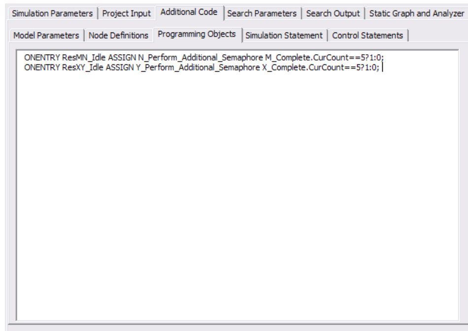
Figure 8.34 Additional code stipulating ResMN's working sequence from M1 to M5 and then N1 to N5, and ResXY's working sequence from X1 to X5 and Y1 to Y5
