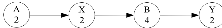
Figure 7.32 Indirectly dependent resource-sharing Activities X and Y with a slower-production-rate Activity B between them
