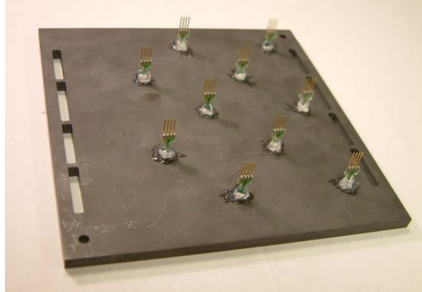
Figure 3-3: A flow field plate embedded with RH sensors
