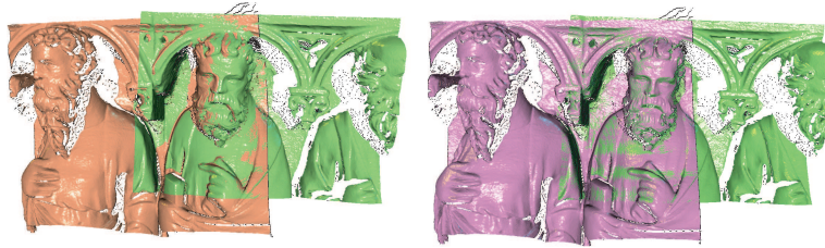
Figure 1.8: Surface matching for surfaces with partial overlapping. A and B: two scanned surfaces from Arrigo data set; C: the relative position of the surfaces before surface matching; D: result after approximate surface matching; E: refined result after applying ICP.
