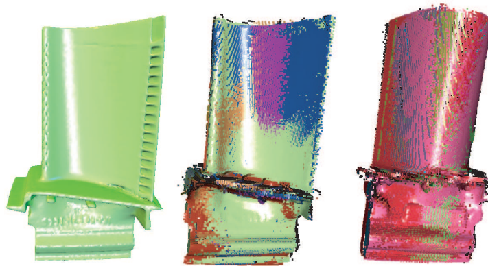
Figure 4.10: Matching result of the Turbine model. Left: the Turbine model. Center and right: 12 scans of the Turbine model after initial matching.
