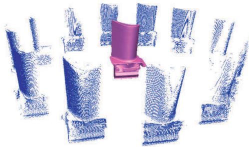
Figure 4.1: Multi-view scans of one object and their nominal CAD model. The CAD model of Turbine Vane is shown in the middle. Twelve scans obtained from a manufactured Turbine Vane are shown from corresponding points of view.
