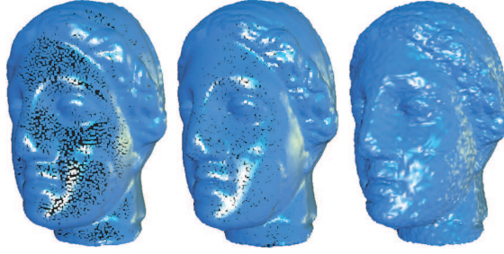
Figure 2.1: Examples of surface variations. Original, resampled, and noisy datasets for the evaluation of feature point detection stability.
