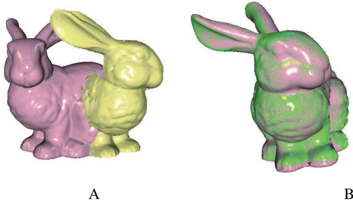
Figure 1.6: Match a scanned surface to its model. A: original position of Stanford Bunny model (purple) and one scanned surface (yellow); B: the result after aligning scanned surface and model.
