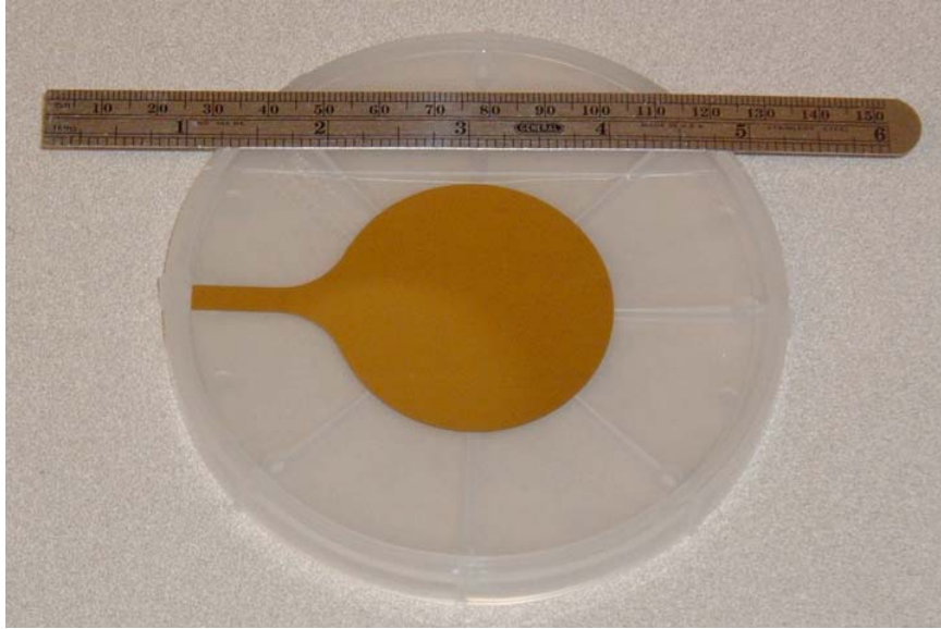
Figure 5.14: Picture of a gold electrode deposited on a glass wafer.
