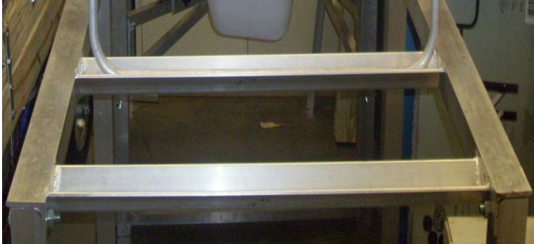
Figure 93: 'V' Shaped Holders for back Support Bar
