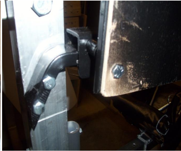
Figure 106: Tablet Arm Attachment to Frame
