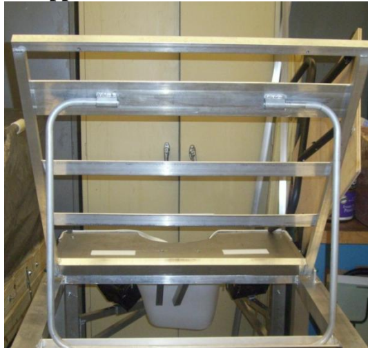
Figure 98: Support Bar on the back of the Back Support
